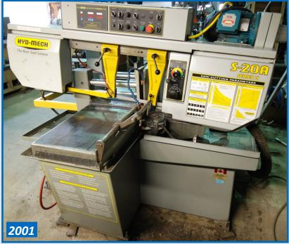
HYD-MECH S-20A SERIES II AUTOMATIC HORIZONTAL BANDSAW
